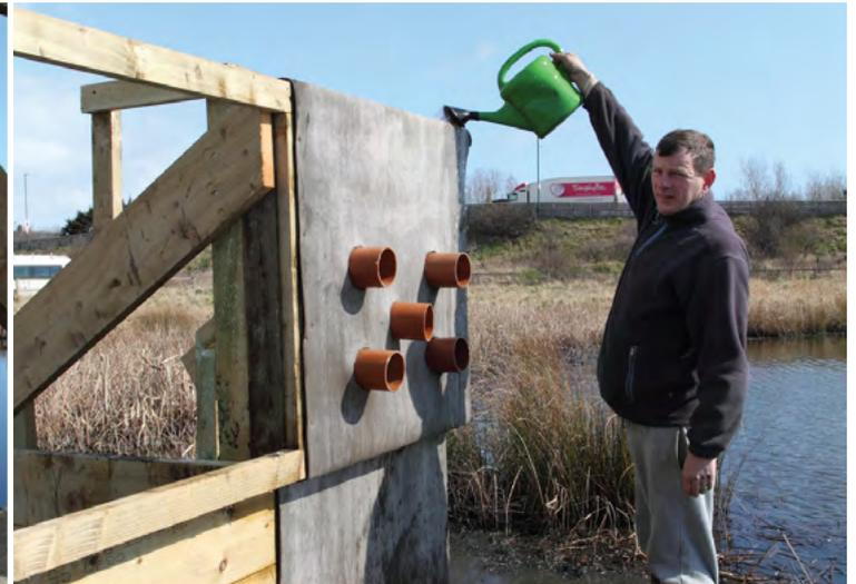
Vertical layer of CC undergoing hydration after insertion of nesting tubes
